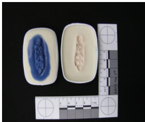
Figura 3b: Chewing gum replication after material cure; notice that the excess material must be removed
