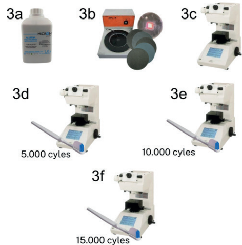
Figure 3 - Methodological Sequence for Microhardness Analysis
